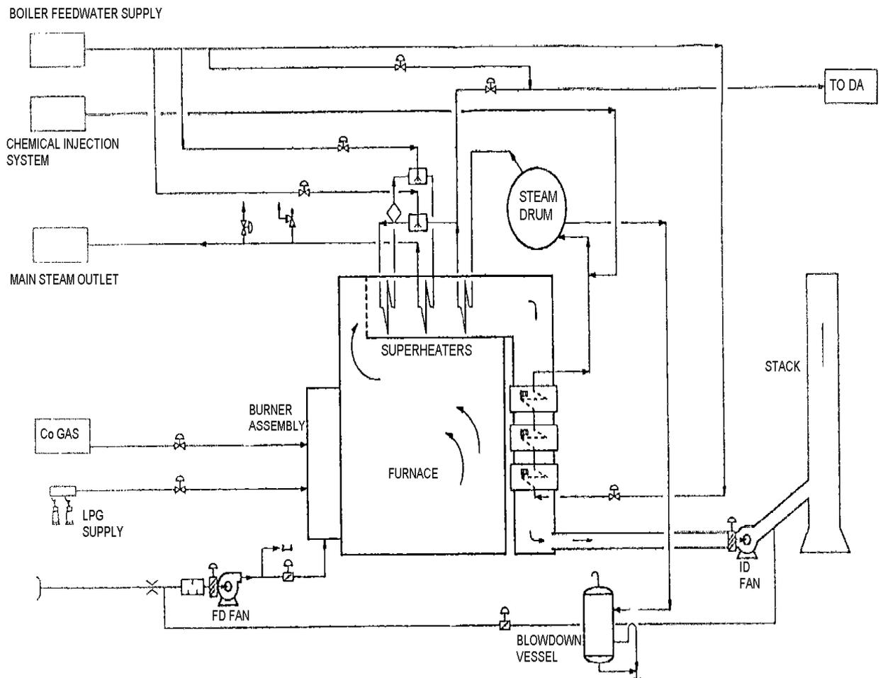
**FIGURE 2 - PROCESS FLOW DIAGRAM OF THE BOILER**
